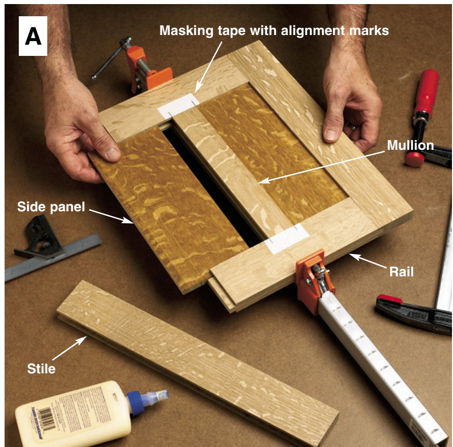
With the mullion and rails assembled, slide in the panels without glue. Glue and clamp the stiles to the rails, keeping them flush at the top and bottom.
